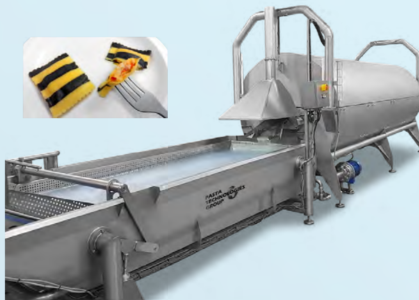
Pre-cooking line for ravioli, capacity 3000 kg/h
