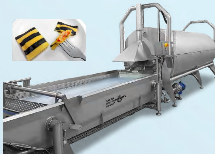
Pre-cooking line for ravioli, capacity 3000 kg/h
