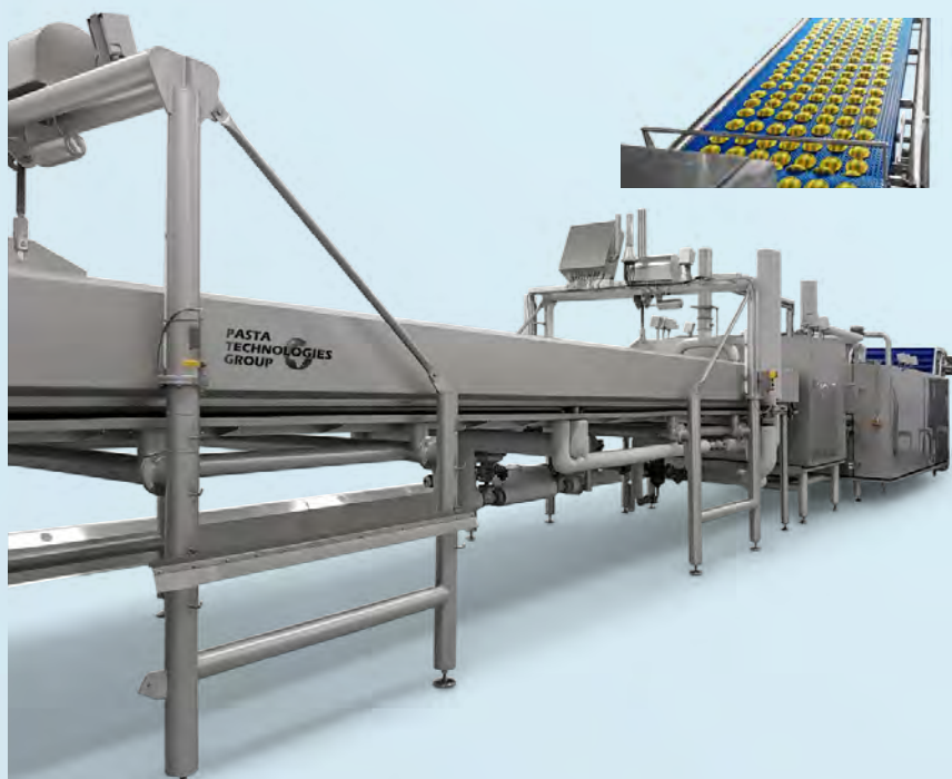
Pasteurized pasta line, capacity 2000 kg/h
