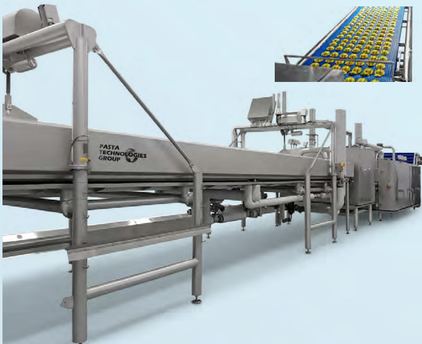
Pasteurized pasta line, capacity 2000 kg/h
