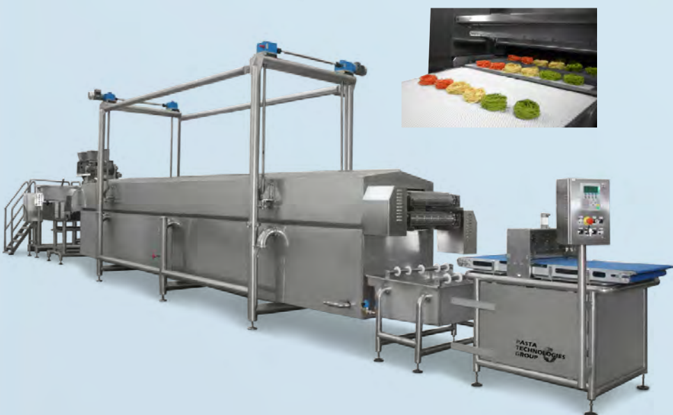
Pre-cooked lasagne line, capacity 800 kg/h
