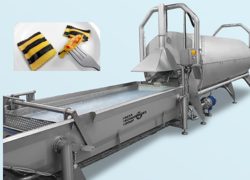
Pre-cooking line for ravioli, capacity 3000 kg/h
