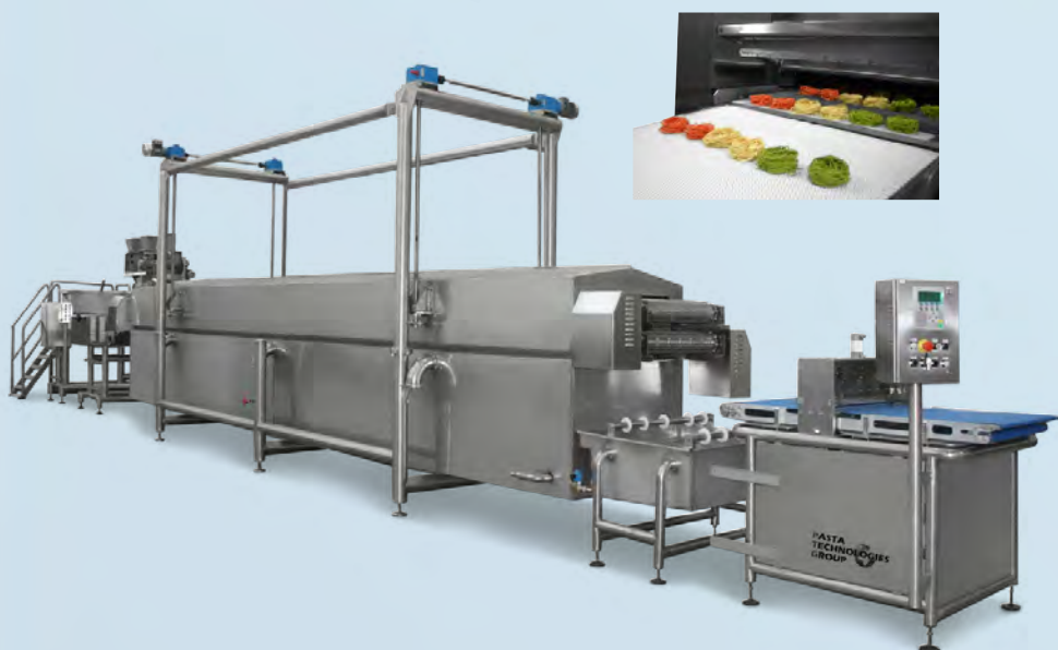
Pre-cooked lasagne line, capacity 800 kg/h
