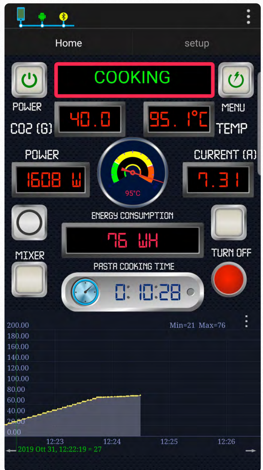
Figure 2 PHOTO OF THE APPLICATION INSTALLED ON A MOBILE PHONE WITH BUTTONS, WINDOWS AND GRAPHS SHOWING THE COOKING TEMPERATURE AND ENERGY OUTPUT DURING PASTA COOKING
