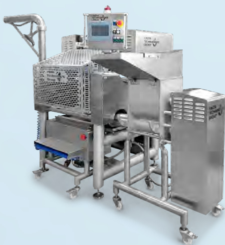
CAPPELLETTI MACHINE MOD. FA630 WITH SCREW PUMP FOR TRADITIONAL FILLING. Available in several models.
