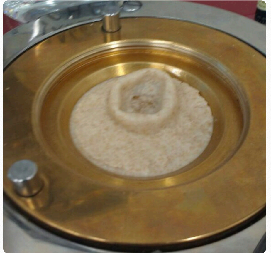
Figure 3 IMAGES OF SENATORE CAPPELLI SEMOLINA (LEFT) AND MONOCOCCUM SPELT (RIGHT) DOUGHS DURING ALVEOGRAPHIC TEST
