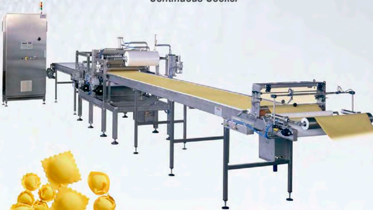
Interfoliatrice Line for sheet with interleaf film
