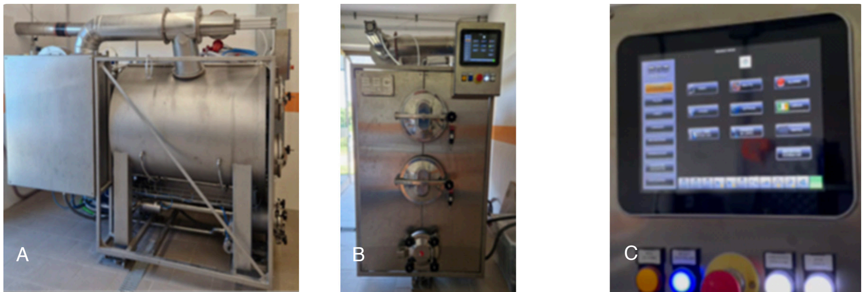
Figure 2 PHOTOS OF THE PILOT MALTING PLANT USED: (A) SIDE VIEW, (B) FRONT VIEW, (C) CONTROL PANEL
