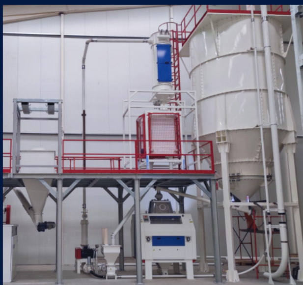
Grinding and recovery of pasta scraps
