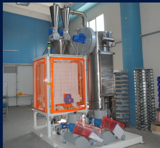
Couscous storage, conveying and selection
