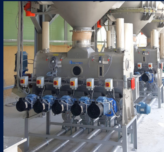
Couscous storage, conveying and selection
