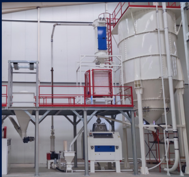
Grinding and recovery of pasta scraps
