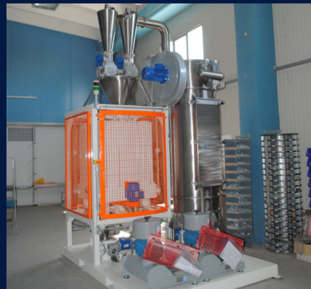
Couscous storage, conveying and selection
