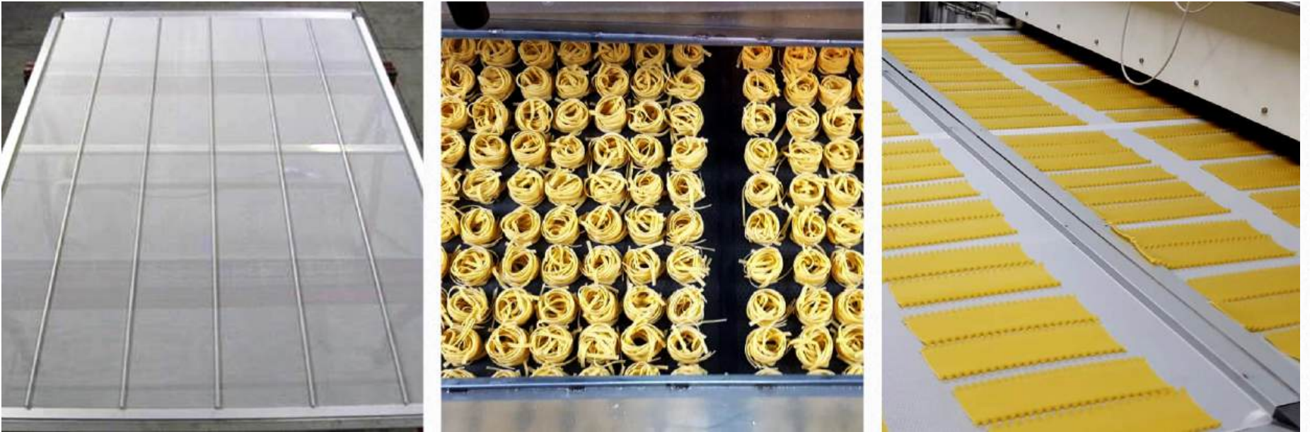
Figure 3 SLATTED TRAYS THAT CAN BE ADAPTED TO THE PACKAGING OF DIFFERENT PASTA SHAPES
